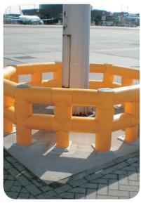
The assembled unit forms a regular polygon with equal side lengths and equal internal angles. All posts are fitted with 225mm OD rotating wear collars to provide enhanced impact and absorption properties and the two horizontal side rails have impact height centres of 310 and 660mm.
